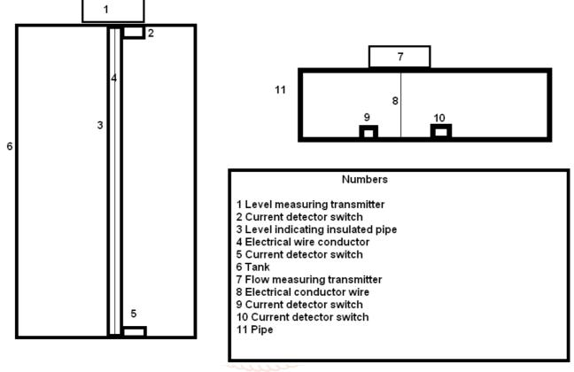
**Construction equipments:** Level and Flow transmitters, Current detector switches, Electrical wire conductors
