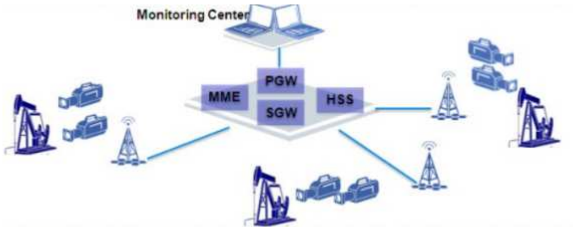
Figure 4 An LTE network for video monitoring [8].
