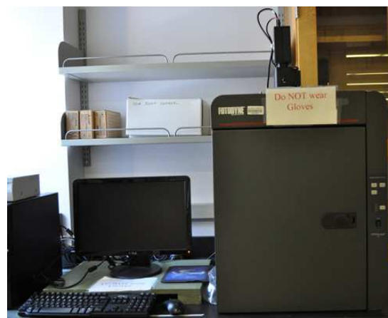
Figure 4. An example of a gel documentation system.
