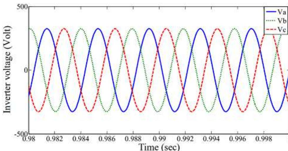
**Fig.5.25. Three phase PWM inverter voltage**
