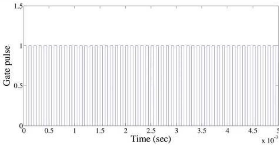
**Fig.5.14. Generated PWM signal for the boost converter**
