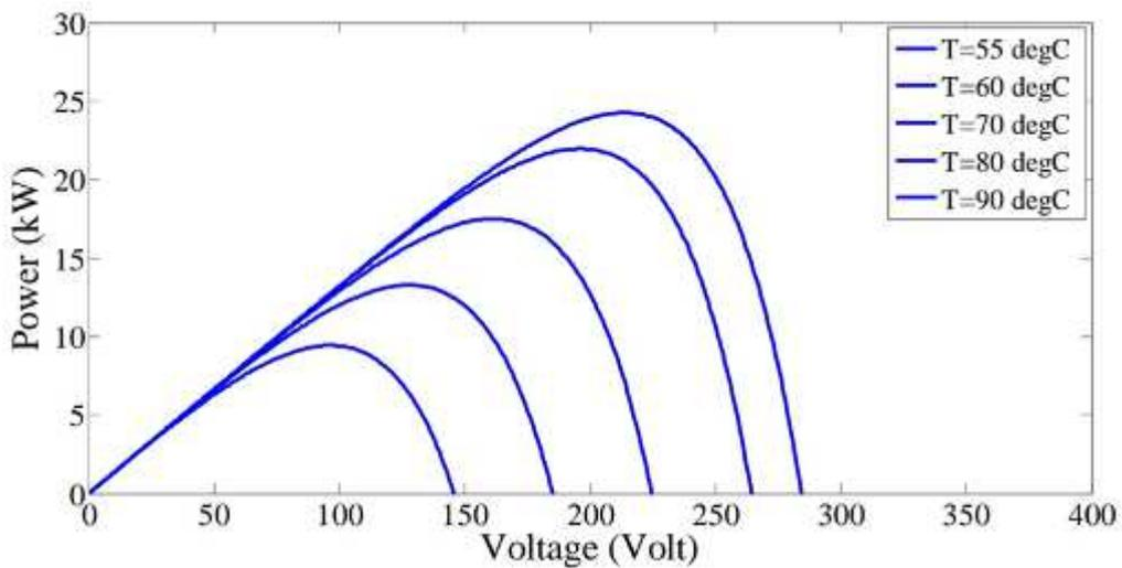
**Fig.5.3. P-I output characteristics of PV array for different temperatures**
