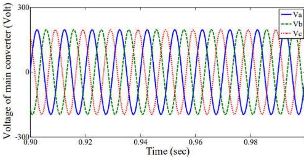
**Fig.5.21. AC side voltage of the main converter**
