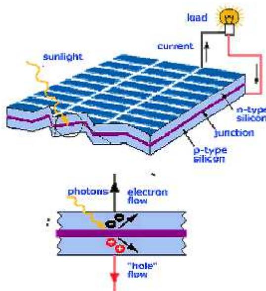
Fig.3.1. Basic structure of PV Cell
