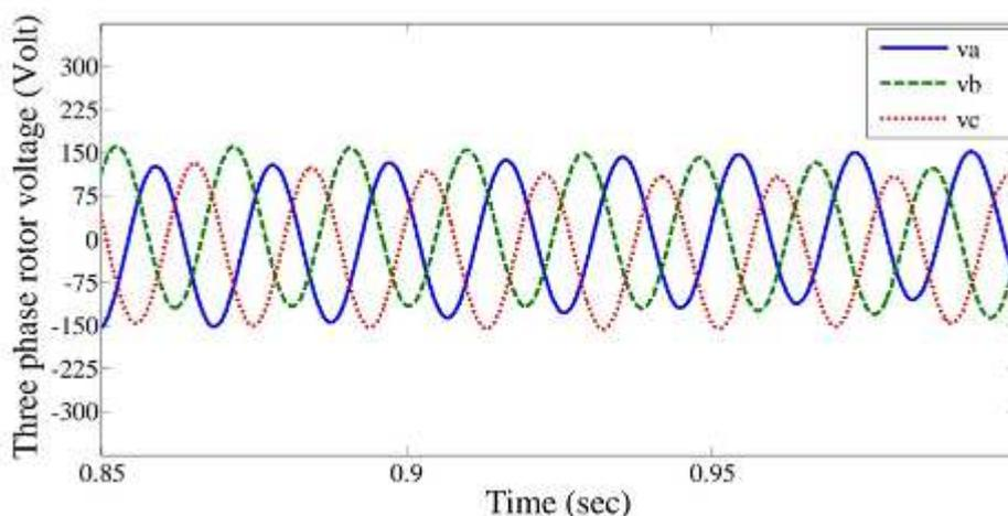
**Fig.5.9. Three phase rotor voltage of DFIG**
