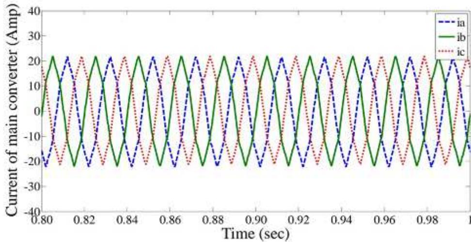
**Fig.5.22. AC side current of the main converter**
