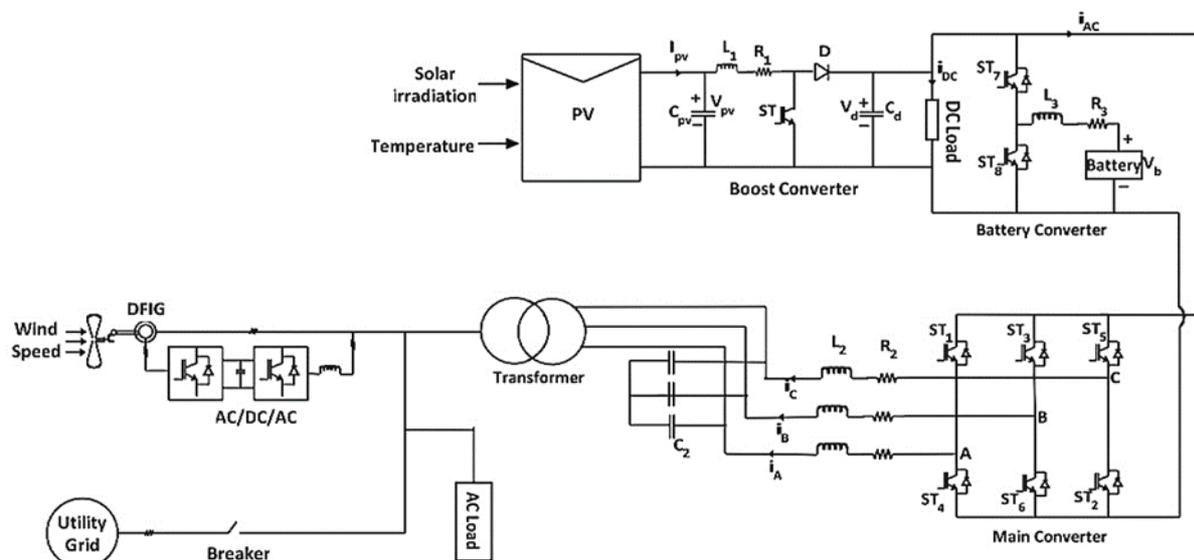
**Figure 4.2 describes the hybrid system configuration which consists of AC and DC grid.**
