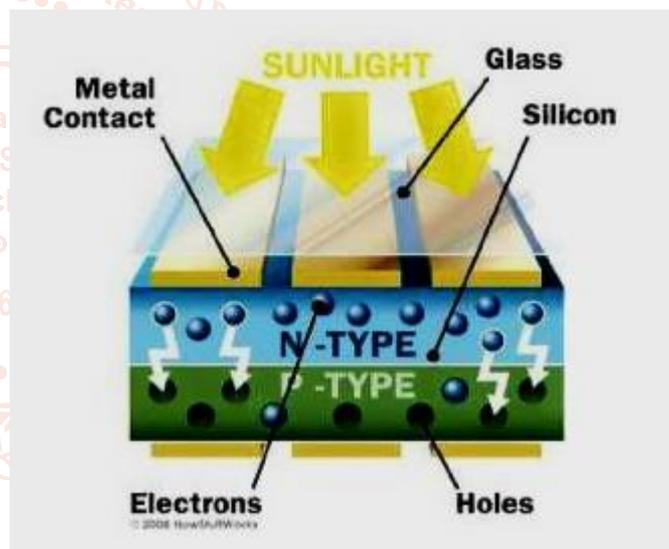
**Fig.3.3. Working of PV cell**
