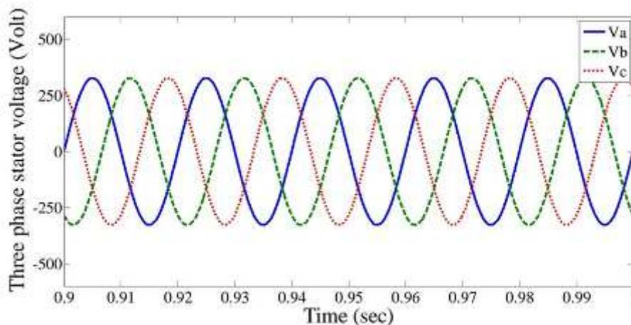
**Fig.5.8. Three phase stator voltage of DFIG**
