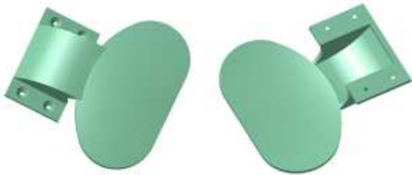
Figure No. 1 3D model of Pressure Die Casting for Door Handle
