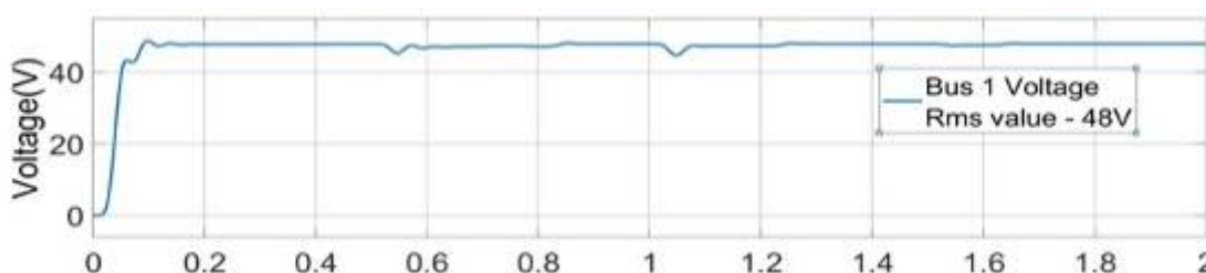
Fig.16 waveform of bus1 voltage
