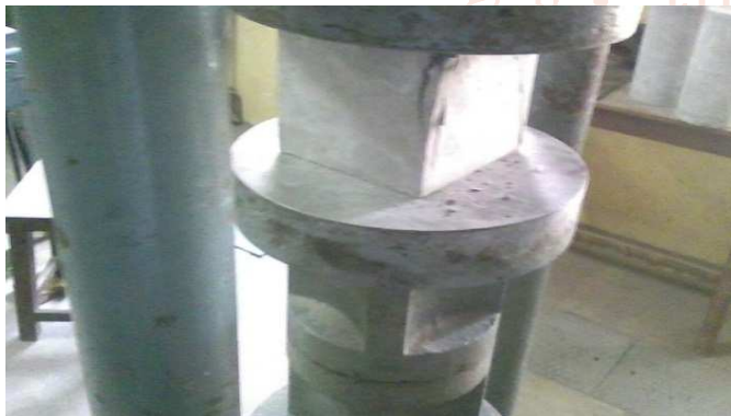
Fig 4.4 Experimental setup for Compressive Strength
