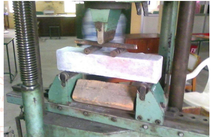
Fig 4.7 Testing of concrete beams specimens
