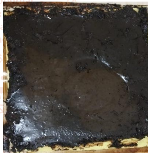
Sample 4 CNSL resin with 5: 1 ratio with catalyst
