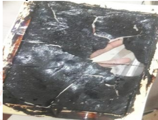
Sample 2 CNSL resin with 3: 1 ratio
