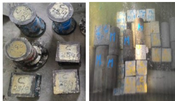
Fig 4.3 Casting and Curing of Specimens
