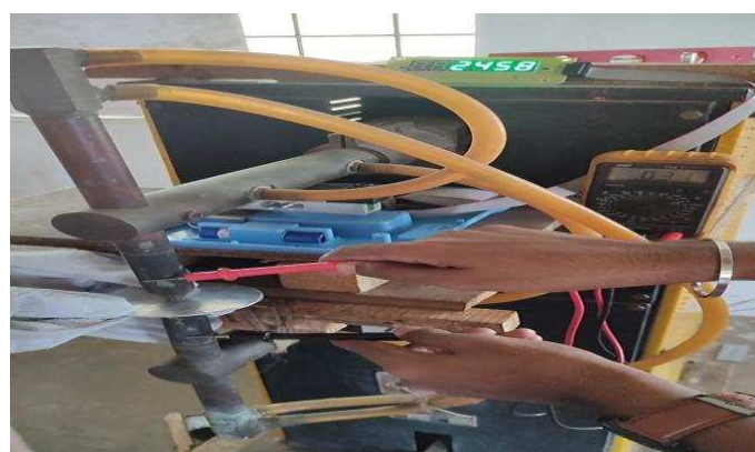
Figure 4 Spot welding with load cell
