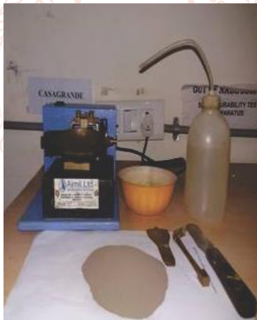
Fig.4.7 Experimental setup for determination of liquid limit
