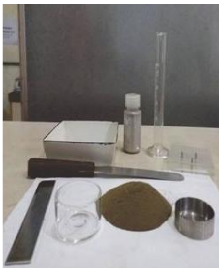
Fig.4.9 Experimental setup for determination of Shrinkage limit of specimen
