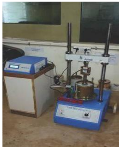
Fig.4.12 Experimental setup of CBR test of specimen
