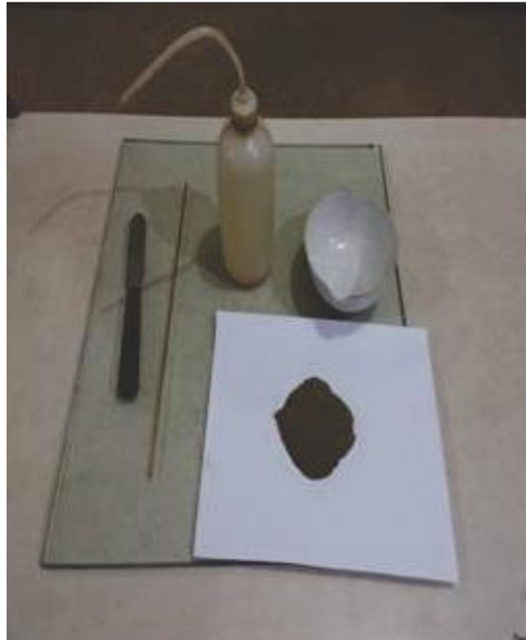
Fig.4.8 Experimental setup for determination of Plastic limit
