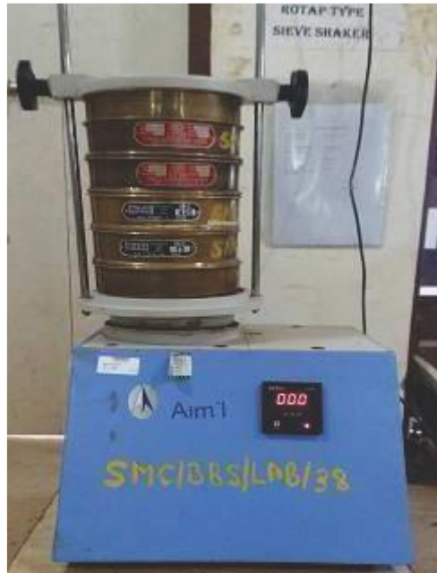
Fig.4.6 Sieve analysis in progress
