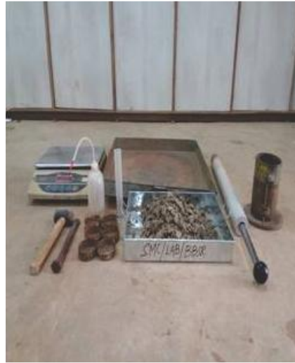
Fig.4.11 Experimental setup of compaction test of specimen
