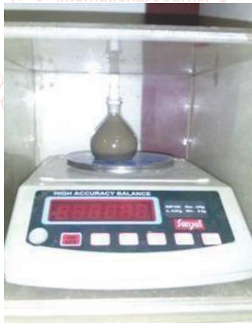
Fig.4.7 Specific gravity test in progress
