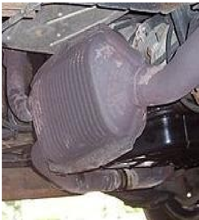
Figure 1 A three-way catalytic converter
