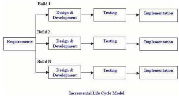
**Figure 4.3: Iterative and incremental methodology**
