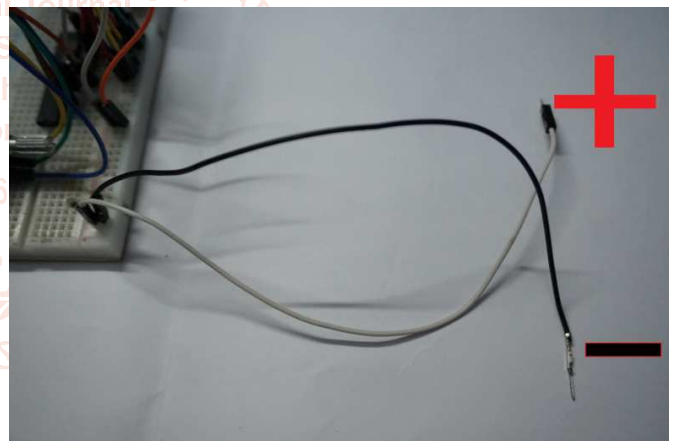
Figure 24: Power supply wires.
