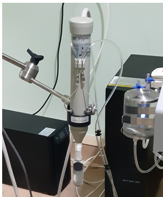
Fig. 2 Ultrasonic transducer for HIFU therapy, filled with degassed liquid.
