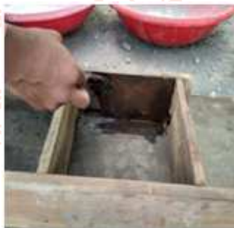
Fig 4.3 Oil coating on mould
