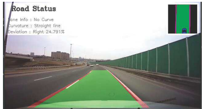
Fig 8 lane detected on the input video
