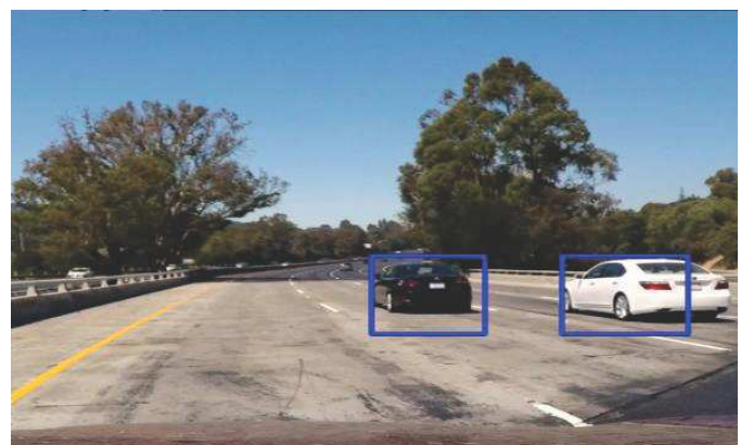
Fig 11 Detected and Tracked vehicle
