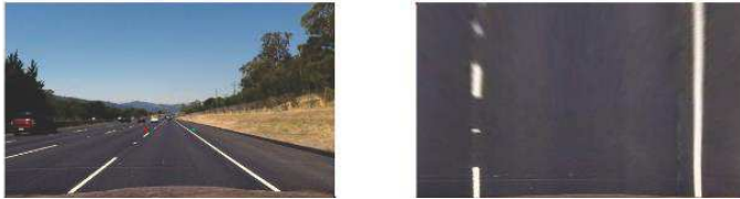
Fig 6 perspective transformation of the original image
