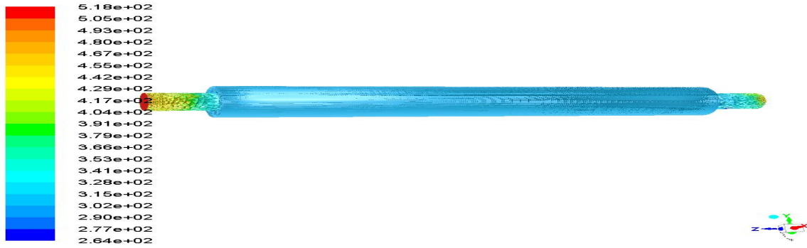
Figure 13 at a brake power of 3.08 KW, PFCHE with triangular fin temperature contour
