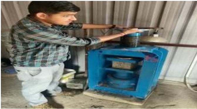
Figure.4.6 Compressive Strength test
