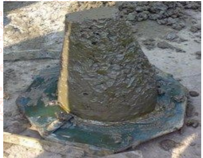
Figure 4.5 Slump cone test
