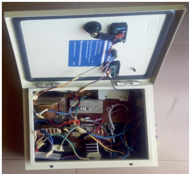
Fig.5. Inner view of the open casing unit of the completed inverter circuit
