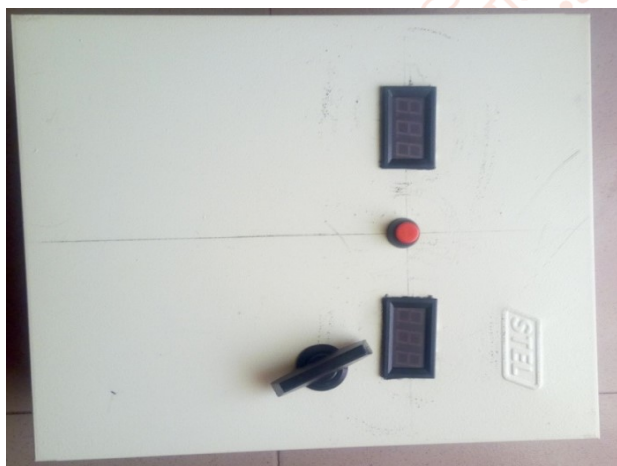
Fig.6. Top view of the sealed metal casing unit of the completed inverter circuit
