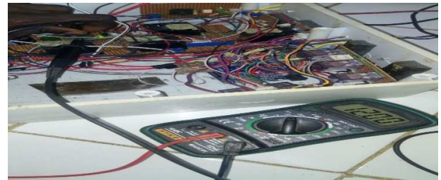
Plate 1: 7812 voltage regulator output voltage
