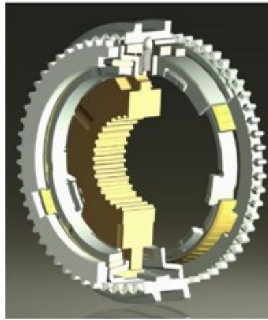
Cross-Sectional view of Single Cone Synchronizer
