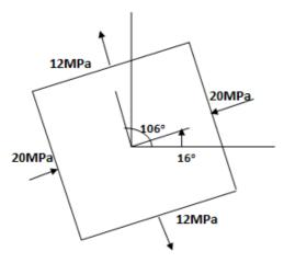
In this way we can calculate the principal stresses and angles at which the principal stresses act by matrix method.
