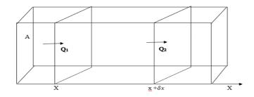
Hence, the quantity of heat  $Q_1$  flowing into the section at a distance  $\boldsymbol{x}$  will be
