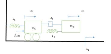
Transfer function: It is the relation between the output and the input of a dynamic system written in complex form (s). For a dynamic system with an input u(t) and an output y(t), the transfer function H(s) is the ratio between the complex representation (s) of the output Y(s) and input U(s).
