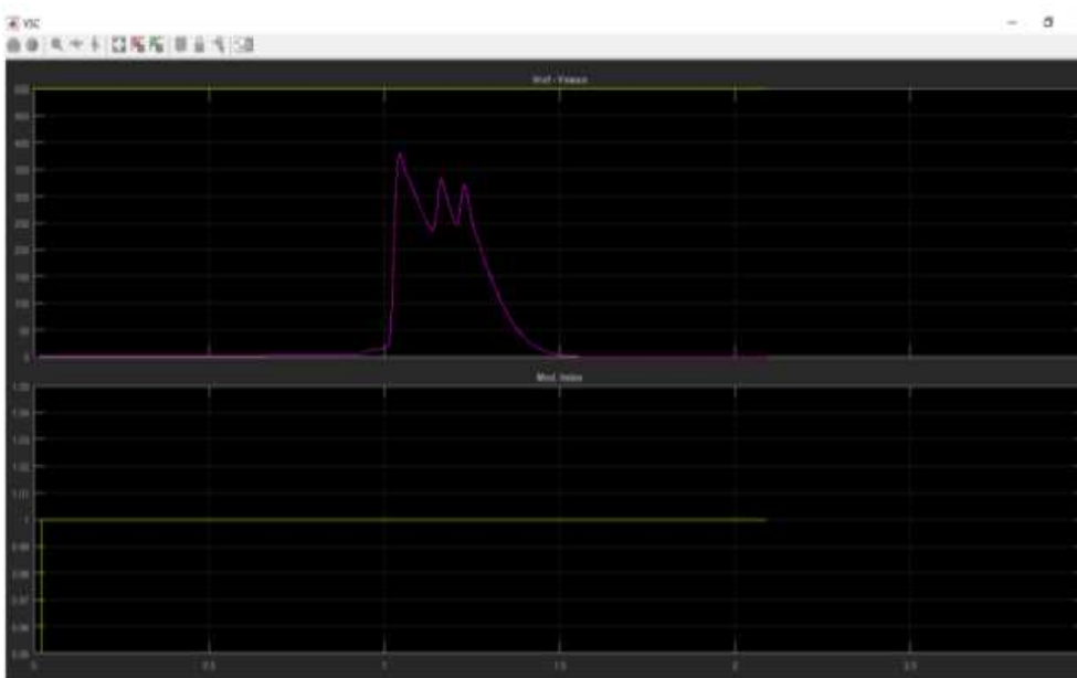
Figure 1.8: Out Characteristics of Voltage Source Converter (VSC)
