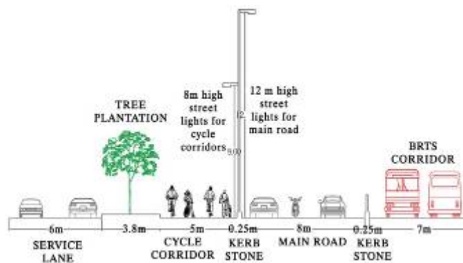
Figure 2- Section of road one way. Source- Author
