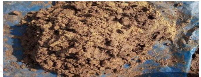
Fig.2 Mixing of Clay Sawdust with Jaggery Mixer
