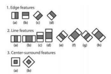
Feature Extraction Haar Cascades use machine learning methods in which a function is trained from a lot of positive and negative images. This process in the algorithm is feature extraction.
