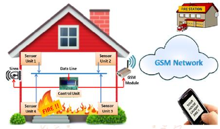
The hardware of the system principally includes detector section, management unit, network module, and power supply
