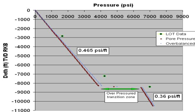
**Figure 7 - Pore Pressure Profile**
