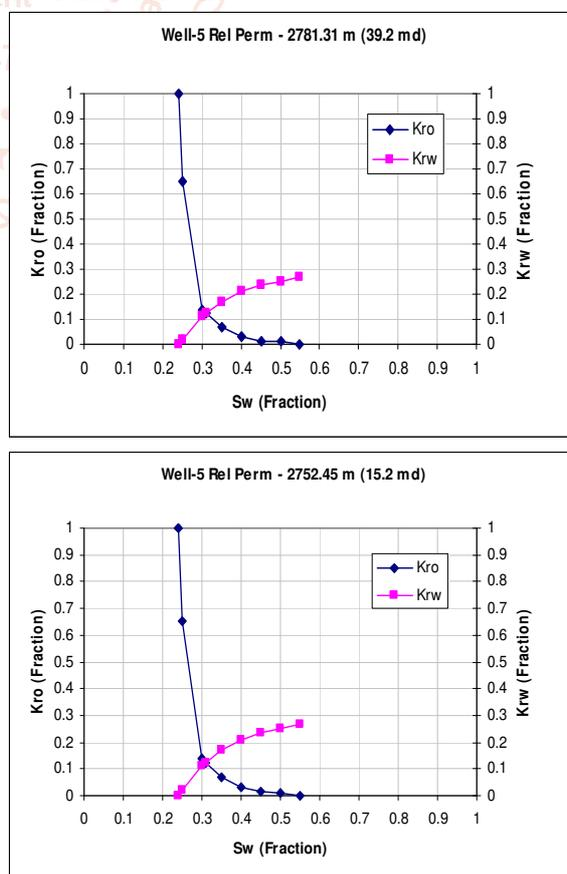
Figure 4 – Rel Perm Curves from SCAL experiments in Well Beta-5
