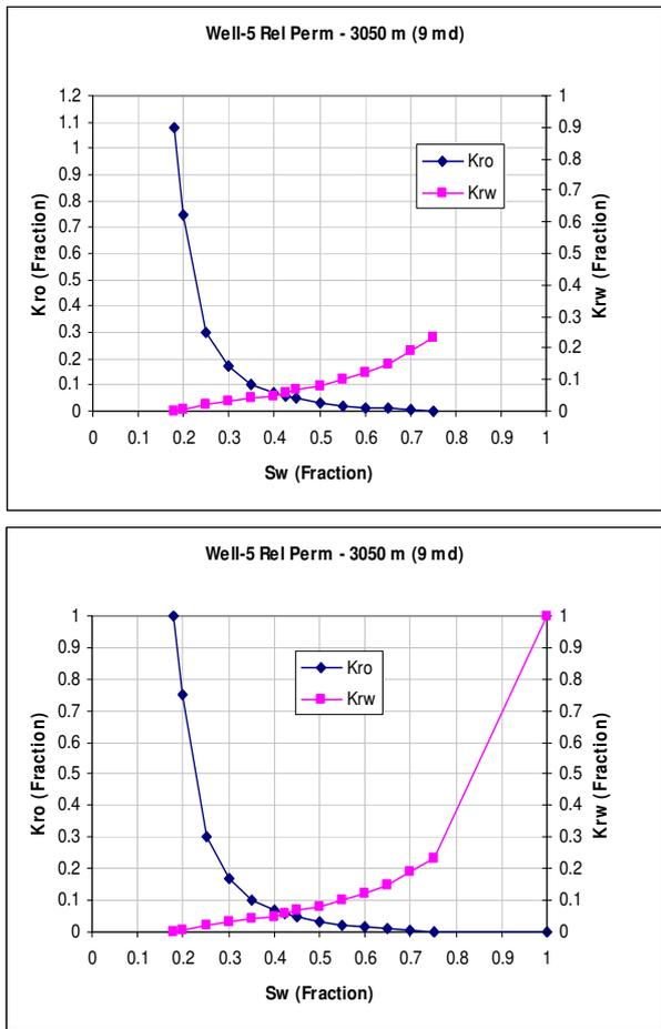
Figure 5 – Rel Perm & Modified Rel Perm Curves for the most Representative Sample.
