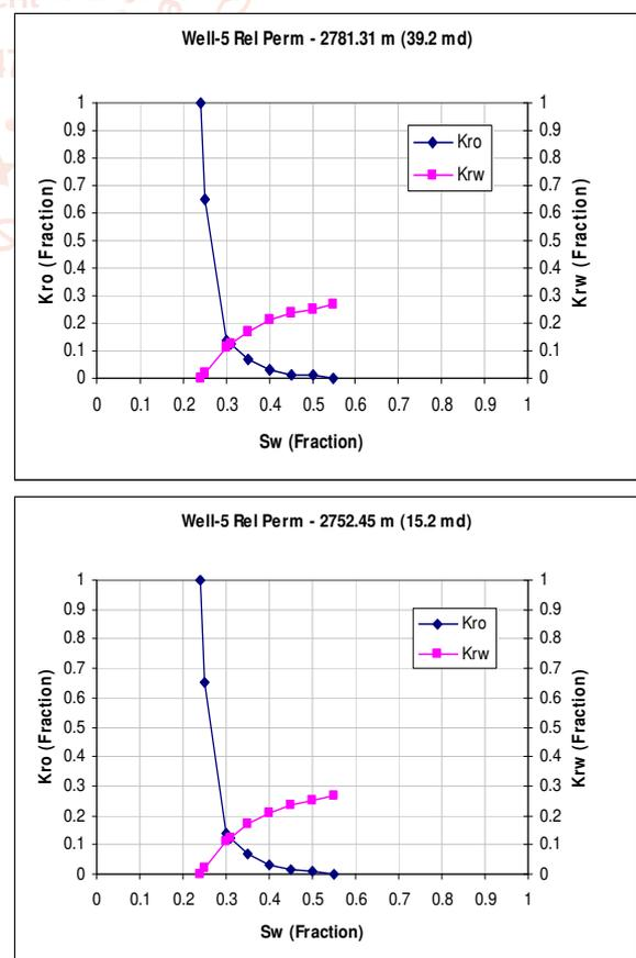
Figure 4 – Rel Perm Curves from SCAL experiments in Well Beta-5
