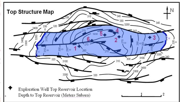
**Figure 3 - Top Structure Map with Highlighted "Known Area"**
