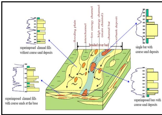
**Figure 2 - 3D Braided River with sedimentary logs. Ref W. Beta-9**
