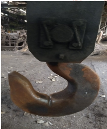
Fig 2: Hook Block of 75 Tonne EOT Crane (BSP, SAIL)
