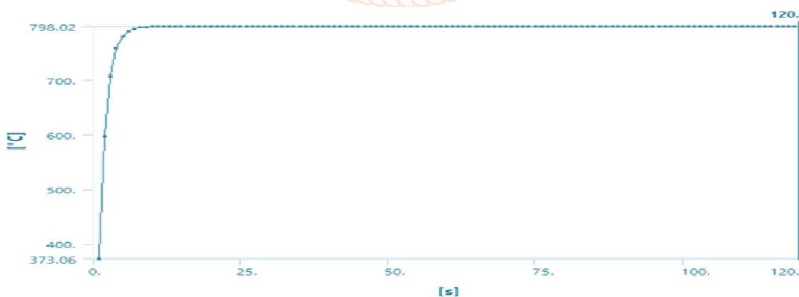
Figure 13 Temperature distribution over time for circular fin with hexagonal hole for step end time 120s
