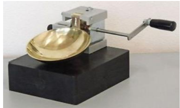
Fig-3 Casagrande's Liquid Limit Device
