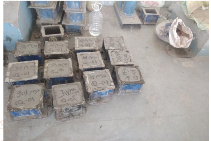
Figure 3 Casting of Concrete Cubes and Beams
