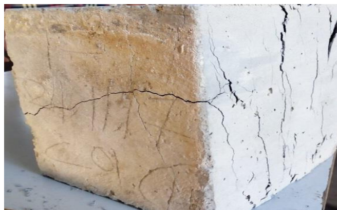
Figure 4. Cracks developed in the bacterial concrete
