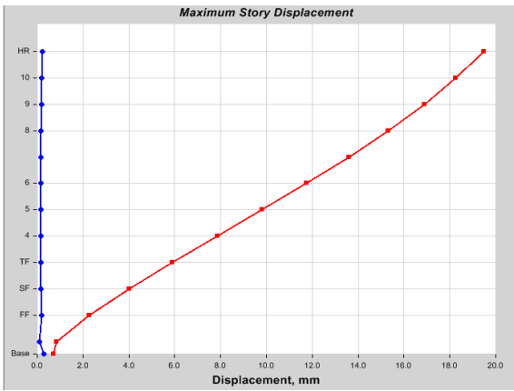
Max story displacement Load Case Earth Quake Y - direction
