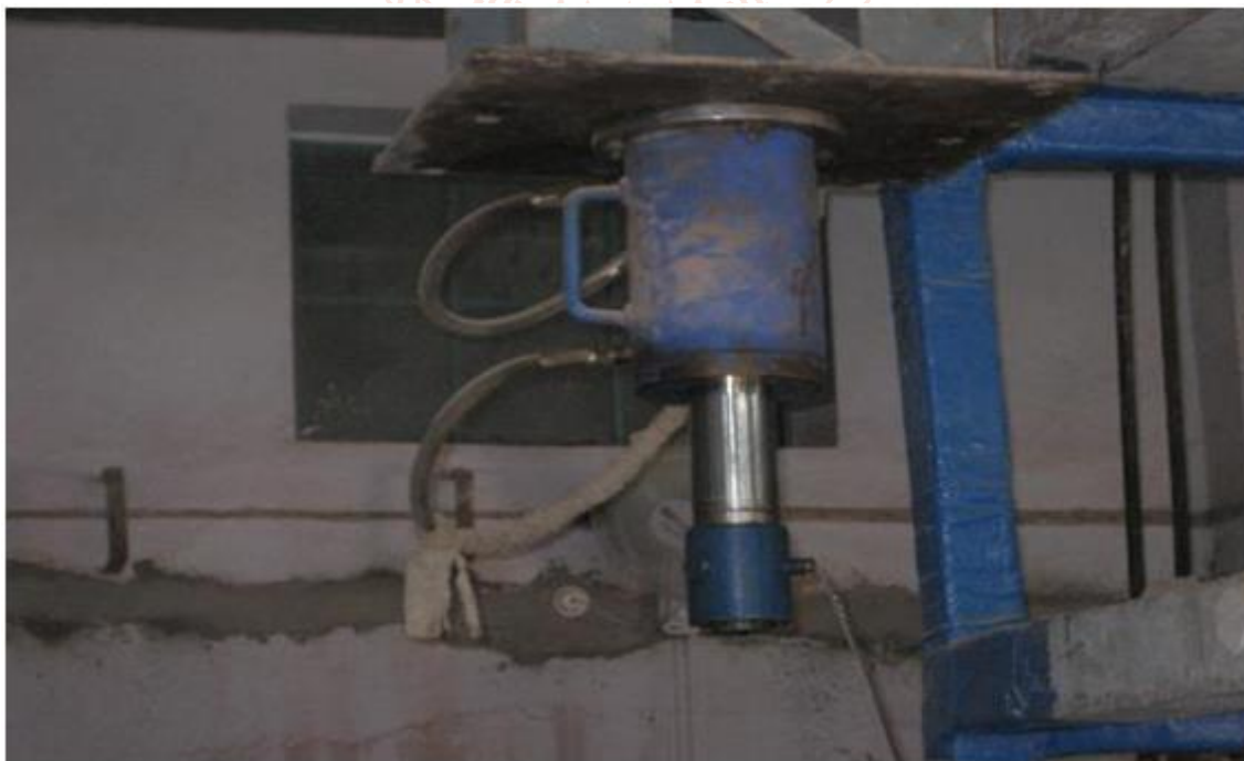
FIGURE 3.4: TESTING JACK SHOWING FULL TRAVEL OF THE JACK
