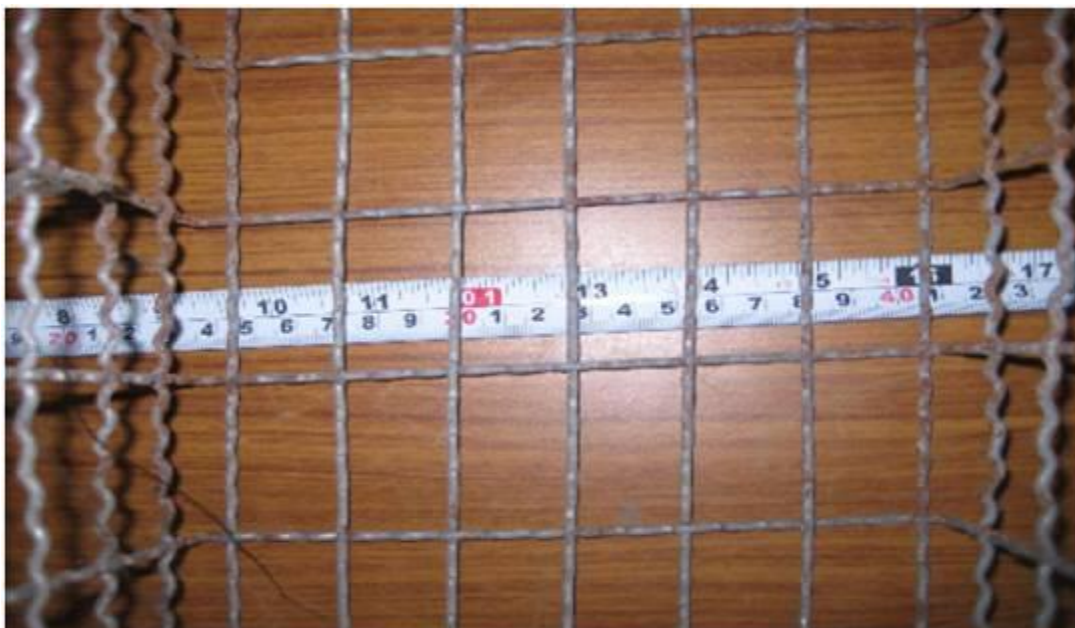
FIGURE 3.10: STEEL MESH SHOWING TRANSVERSE DIMENSION
