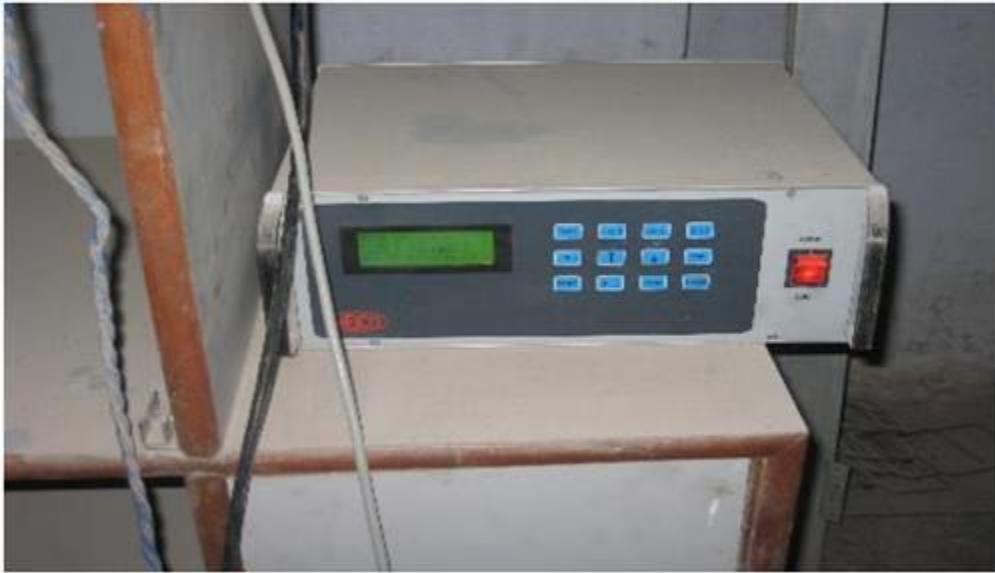
FIGURE 3.5: DATA ACQUISITION SYSTEM CONNECTING WITH LOAD CELL
