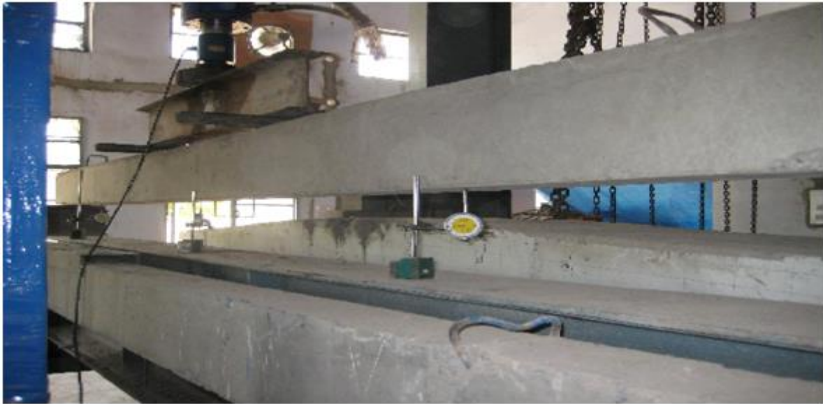
FIGUR 3.11: EXPERIMENTAL SET UP SHOWING POSITION OF DIAL GAUGES
