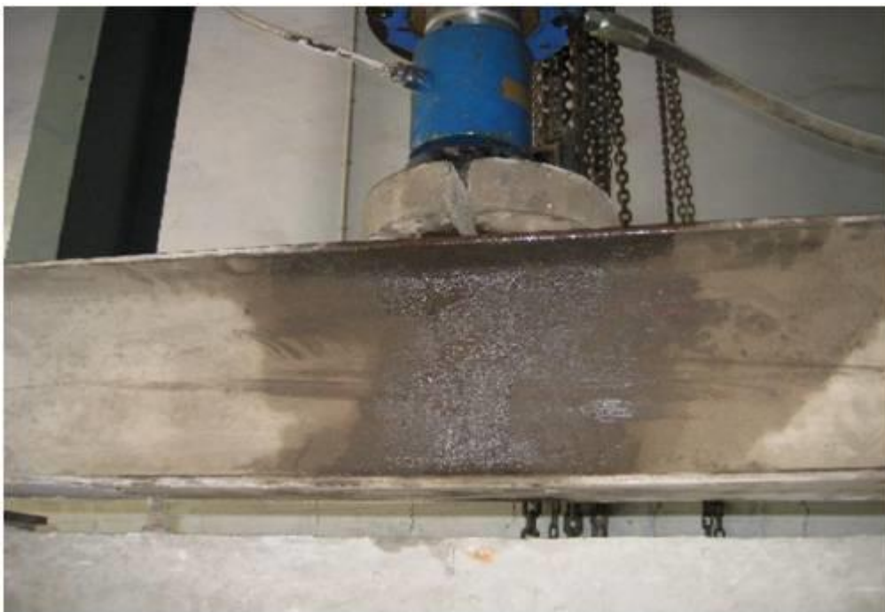
FIGURE 3.6: TESTING JACK WITH SYSTEM FOR CONVERTING CONC. LOAD TO TWO POINT LOAD
