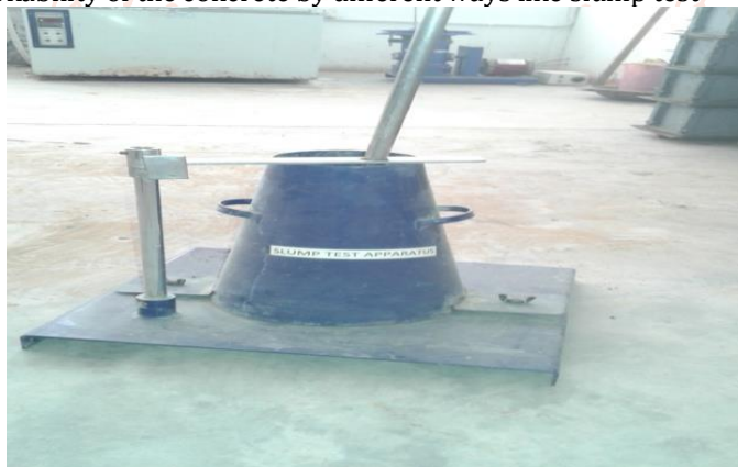
Slump Testing Apparatus
