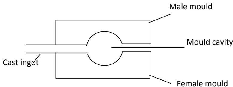
**Figure 3.3: Schematic Diagram of the Mould**
