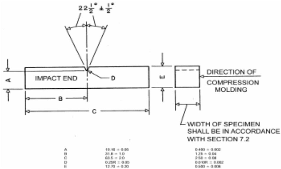
Figure 3.7: Dimension of Izod Test Specimen in ASTM D256
