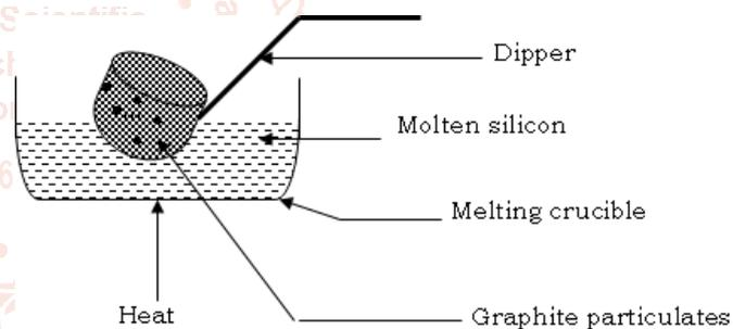
Fig.3.1: The dipping process.
