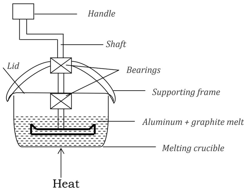
**Figure 3.2: Melting Furnace with Stirring Device**
