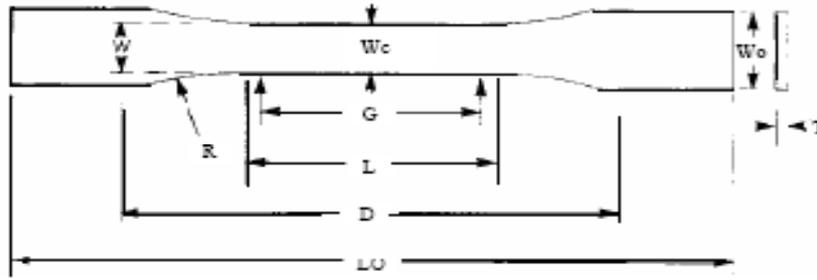
Figure 3.4: Dumbbell Shaped Specimen [ASTM (D638)]
