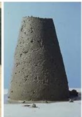
Test Fig 4.2 Slump
