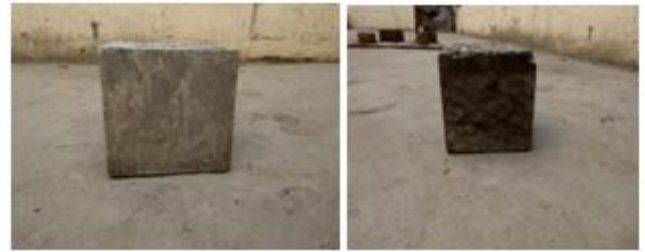
Conventional concrete Light weight concrete Fig 4.5 Specimen for Compressive Strength
