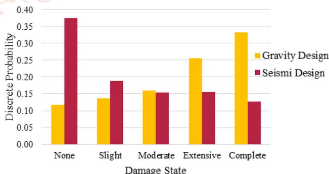
Figure 12. Discrete Probabilities of Different Damage States for Gravity Design and Seismic Design at DBE Hazard level
