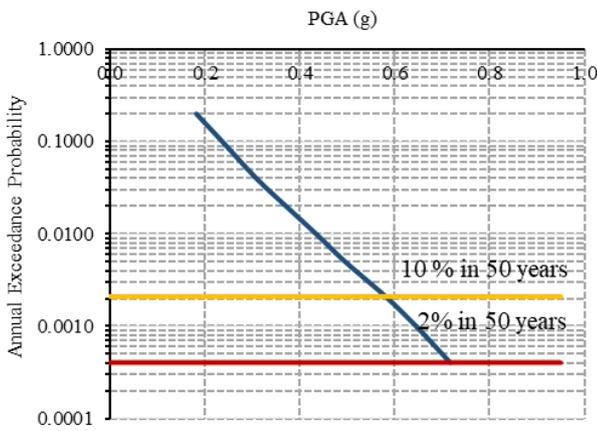
**Fig. 18 Seismic Hazard Curve**
