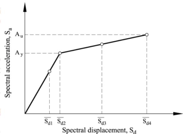
Figure 5. Damage State Thresholds from Capacity Spectrum
