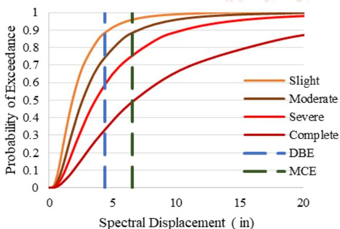
Figure 10. Fragility Curve for Gravity Design Model
