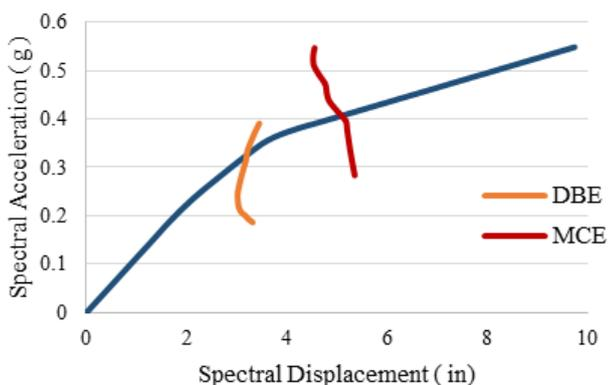
**Figure 6. Capacity Curve with Demand Curves of Seismic Design Model**
