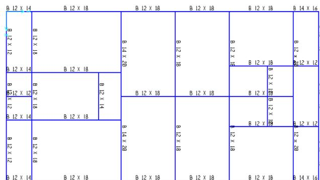
Figure 3. Typical Beam Plan of Seismic Design Model
