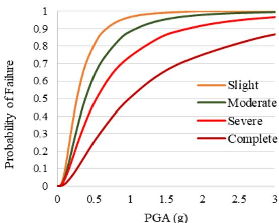
**Figure 14. Fragility Curve for Gravity Design Model**
