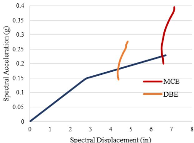
Figure 9. Capacity Curve with Demand Curves of Gravity Design Model
