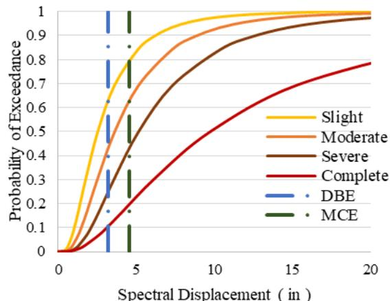
**Figure. 7 Fragility Curve for Seismic Design Model**
