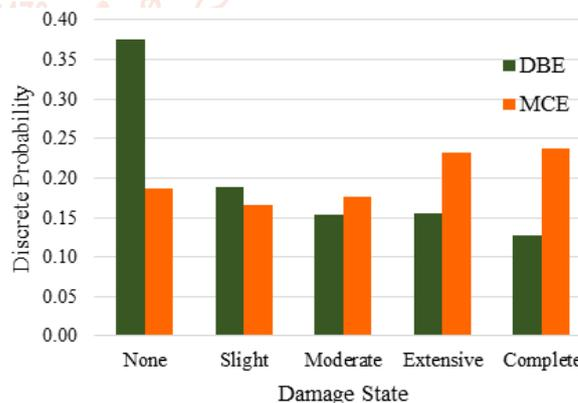
**Figure 8. Discrete probabilities of Different Damage States for Seismic Design Model**
