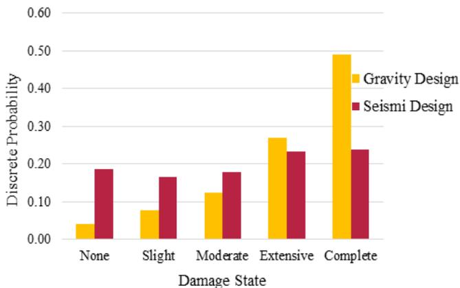
**Figure 13. Discrete Probabilities of Different Damage States for Gravity Design and Seismic Design at MCE Hazard level**
