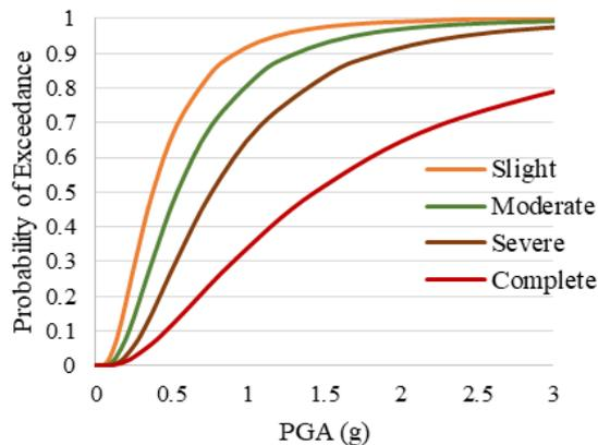
**Figure 15. Fragility Curve for Seismic Design Model**
