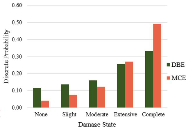
Figure 11. Discrete probabilities of Different Damage States for Gravity Design Model
