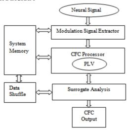
In Block Diagram, Neural signal passes to the modulator. The modulators extracted the samples and send them to the CFC processor. Cross frequency coupling analysis has Phase locking value (PLV) to decrease the period. A system resource has Hilbert filter and Multiplier and counting the data.
