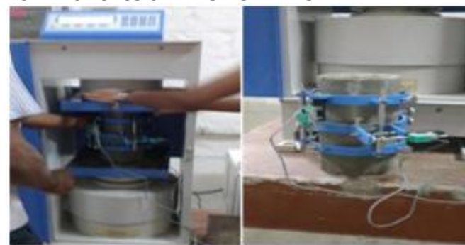
Figure 4.3 Test set up for Young's Modulus
