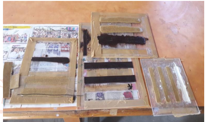
Fig. fabricated composites placed for 24 hours to solidify
