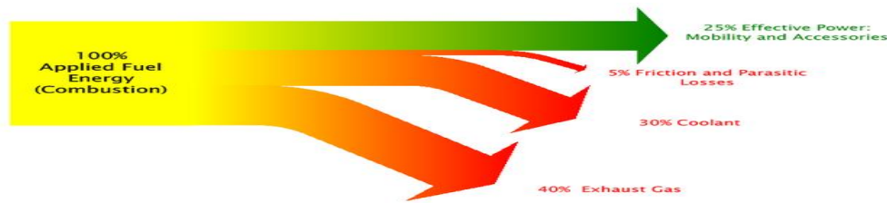
Figure 1 Fuel Energy Distribution of Gasoline Engine.
