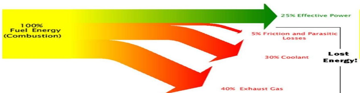
Figure 1 Energy loss in ICEs (internal combustion engines)
