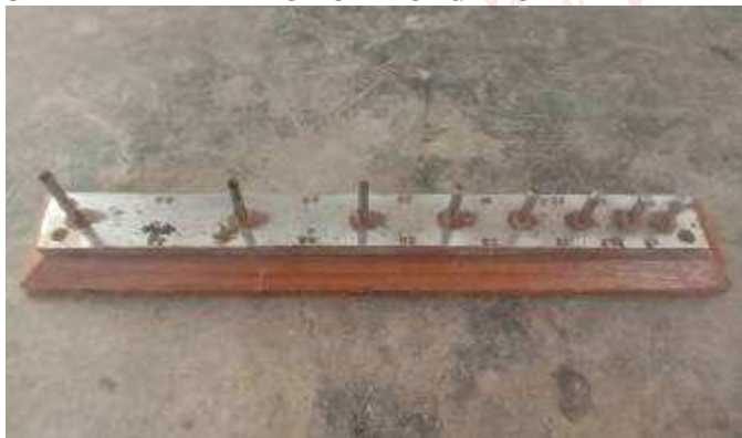
FIG 3.2 ELONGATION INDEX EQUIPMENT
