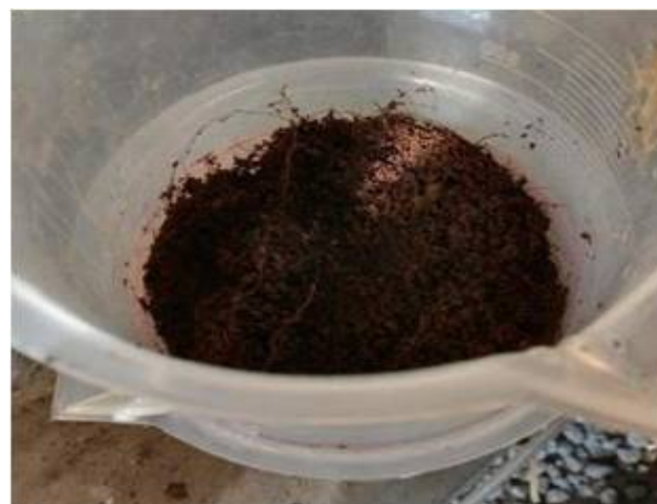
Fig.9. Fibre-mixed Soil Sample brought to OMC
