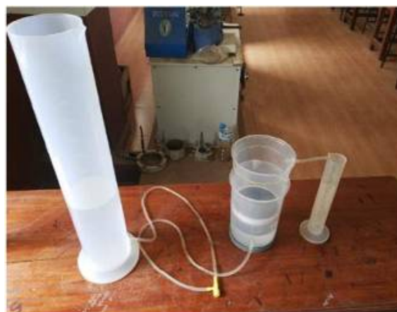
Fig. 7. View of Piping Test Apparatus
