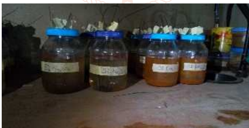
Figure1. Deteriorated/ corroded structural steel and steel sections in sulphate solutions characterized by colored solution
