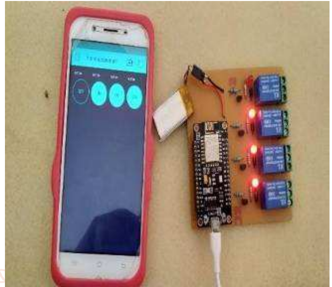
Figure 5: Home Automation System
