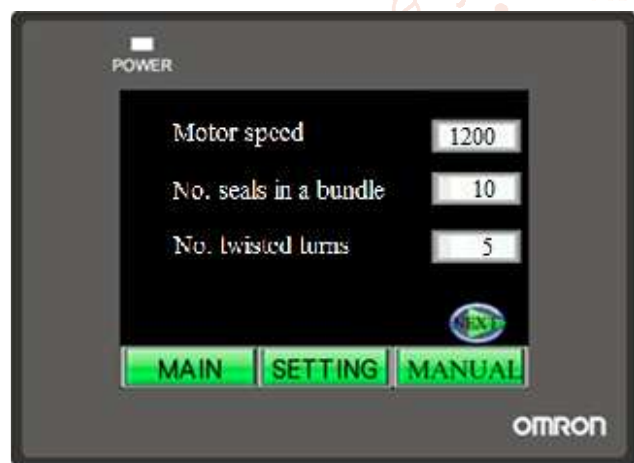
Fig.10. Interface for the program of entering parameters of the wire-winding mechanism
